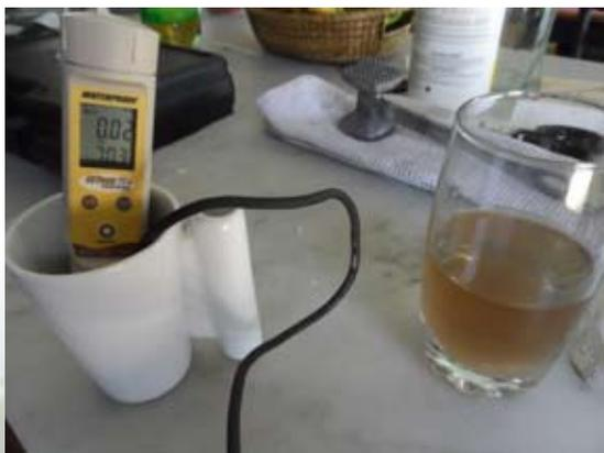
Test reading prior to measuring EC of the VERDE-CAL G. Reading of 0.02 ds/M
